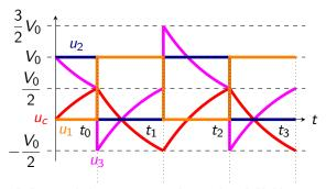
$$u_c = -V_0 + \frac{3}{2}V_0 \exp\left(-\frac{t-t_2}{\tau}\right), \quad u_3 = V_0 - \frac{3}{2}V_0 \exp\left(-\frac{t-t_2}{\tau}\right).$$
