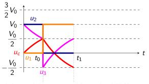
$$u_c = V_0 - \frac{3}{2}V_0 \exp\left(-\frac{t-t_1}{\tau}\right), \quad u_3 = \frac{3}{2}V_0 \exp\left(-\frac{t-t_1}{\tau}\right).$$
