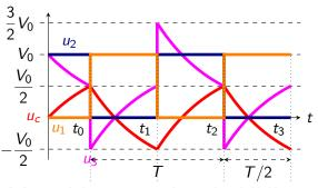
$$-\frac{V_0}{2} = -V_0 + \frac{3}{2}V_0 \exp\left(-\frac{T}{2\tau}\right) \Rightarrow \boxed{T = 2\tau \ln 3}.$$
